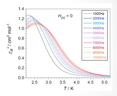
Temperature dependence of the in phase and out-of-phase (right) ac susceptibilities for  $\bf 6$  under a zero applied static field with a  $\pm 3.95$  G oscillating field at frequencies in the range 1000-10000 Hz
