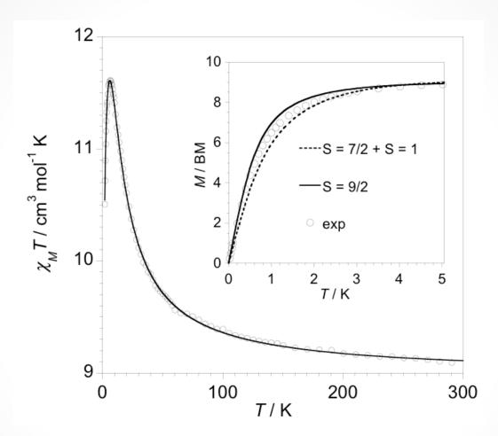
Thermal dependence of  $\chi_{\rm M}T$  for **1**: (o) experimental data, (—) best-fit curve. The inset shows the field dependence of the magnetization at 2.0 K: (o) experimental data; (--) theoretical curve for isolated Ni(II) and Gd(III) ions; (—) theoretical line for an S = 9/2 with g = 2.0)
