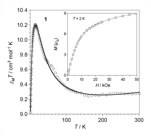
$\chi_{\rm M} T \ vs \ T$  plot for 1: (o) experimental; (—) best-fit curve. The inset shows the magnetization against H plot for 1 at 2.0 K (the dotted line is an eye-guide).
