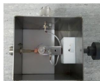
Fig. 11.1 – Measurement cells: a) semi-shielded cells with Copper electrodes; b) MACOR cell shielded with Copper foil; c) metal cell with lid, completely shielded
