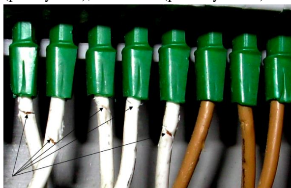
Fig. 7.1 – The effect of aging in less severe exploitation conditions. All conductors from the image are part of one and the same cable; white colored materials show crack (marked by arrows)
