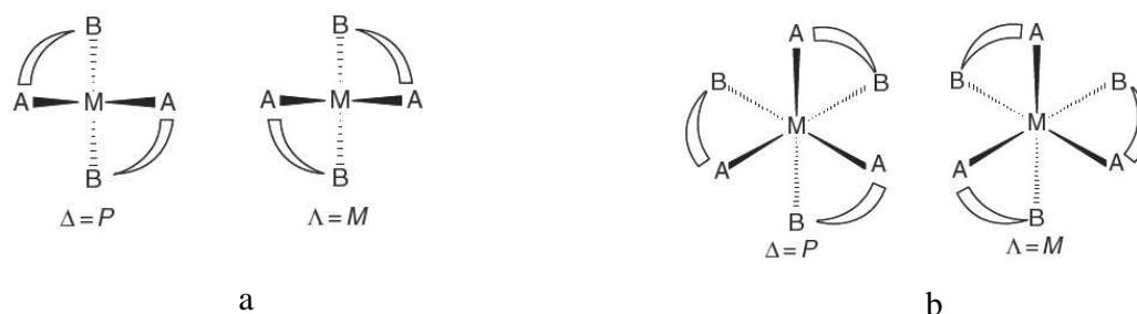
Figure I.32. Absolute configurations and helicities of (a) bis-chelate complexes viewed down the C_2 axis and (b) tris-chelate complexes viewed down the C_3 axis.
